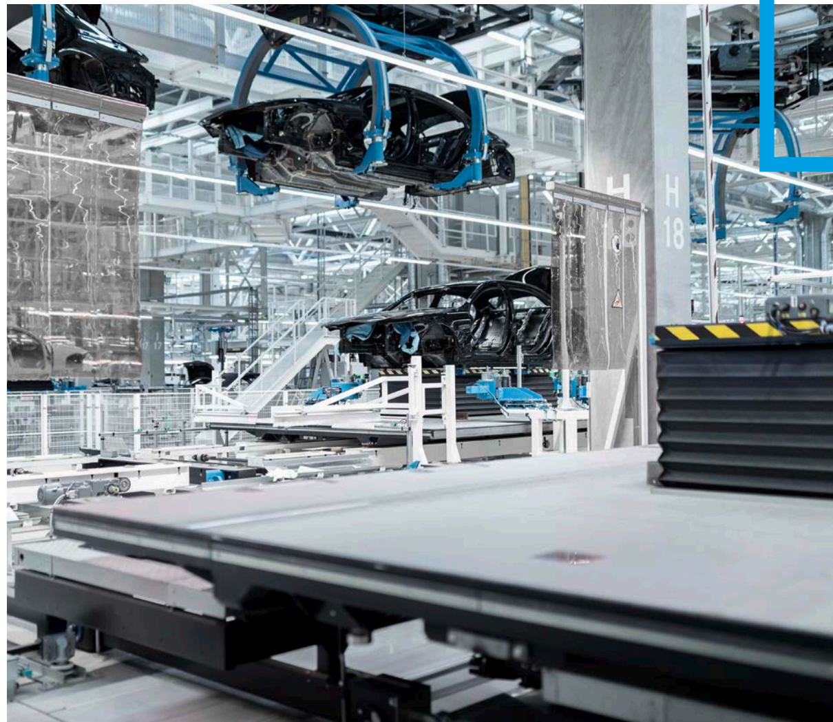
Skillet platform with integrated lift table (bottom right) and heavy-duty EMS with integrated scissor lift (top middle) in a production environment
